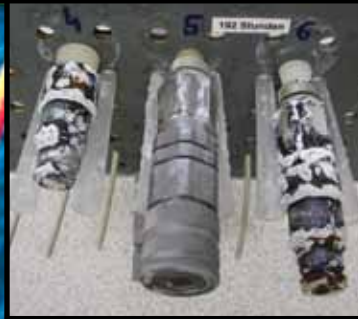
Salt Test at 200 Hours. Holmbury vs Brand A and Brand B
